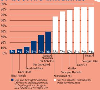
To qualify for an **Energy Star** designation, Republic's roofing products on low-slope applications have met or exceeded the EPA standard of 65% initial reflectivity and 50% reflectivity for three years. Steep slope roofs must have an initial reflectivity of 25% and 15% after three years.
